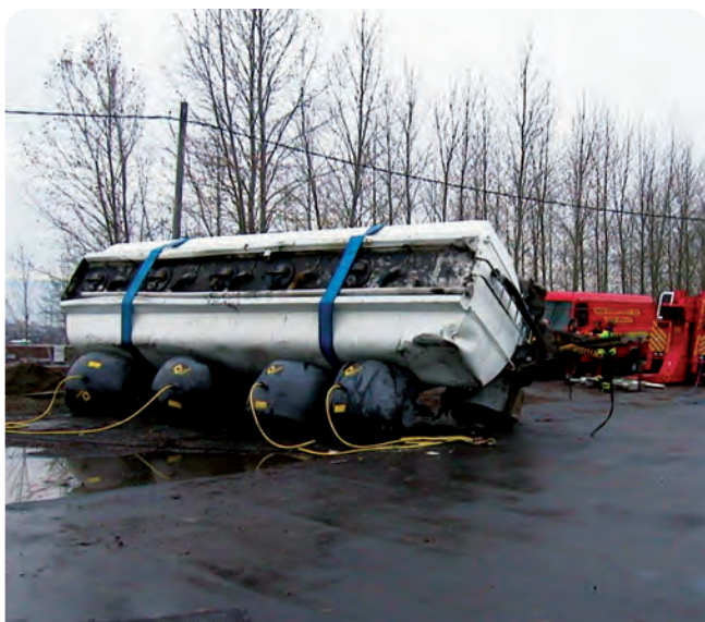
Efficient lifting of overturned vehicles.
